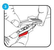
4. Gently pull the audio-lines from the cartridge, taking care to pull from the terminal connector and not the wire itself.
