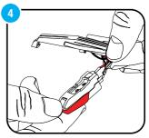
5. Carefully insert the audio-lines into the new cartridge.
