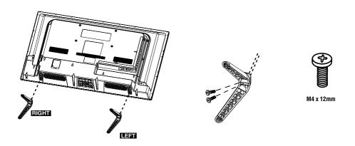
3. Insert the TV stand screws into the designated holes in the rear of the TV base stand and tighten the screws firmly with a Phillips Head screwdriver (not included).
