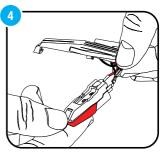
5. Carefully insert the audio-lines into the new cartridge.
