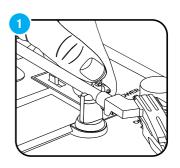
2. Remove the protective cover from the stylus cartridge to expose the needle.
